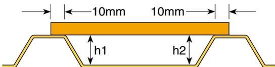
Fig 3: Method for measurement of profile depth
